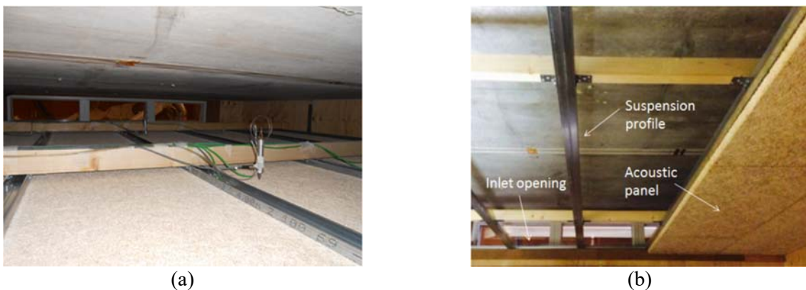
Figure 10: Overhead plenum and diffuse ceiling setup [4]
